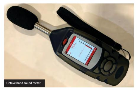
"Most countries recognise noise as a health and safety risk, and as a result, have regulations for noise at work. In the EU a level of 80dBA during the entire working day is seen as the threshold for significant hearing damage in a significant proportion of the population. Therefore, 80dBA is defined in the EU as the working noise level at which action must be taken."
